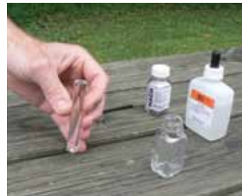
Fill test tube to the top with water sample.
