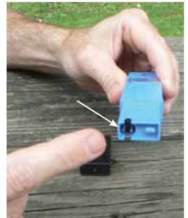
To maintain and improve the performance of your tester clean the stainless steel electrodes on the bottom with isopropyl alcohol.
