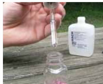
Add Titrant Solution to the mixing bottle one drop at a time while swirling the bottle.
