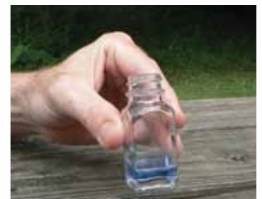
When the color changes from pink to blue, record the number of drops added.
