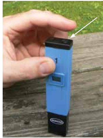
Press the ON/OFF switch once to turn the tester on.
