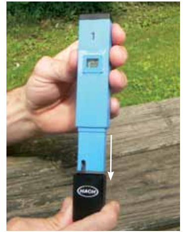
Remove protective cap from the bottom.
